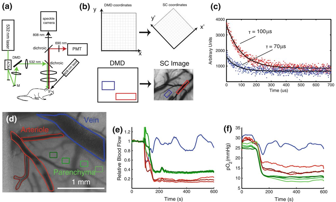
**FIGURE 6.** (a, b) Combined instrument for simultaneous imaging of blood flow and spatial mapping of  $pO_2$ . Spatially resolved  $pO_2$  is obtained by spatially restricting phosphorescence excitation light and utilizing a single element detector to record time-resolved phosphorescence decays (c). (d, f) Measured temporal dynamics of blood flow and  $pO_2$  in eight different spatial regions following stroke induction at  $t = 100$  s.
