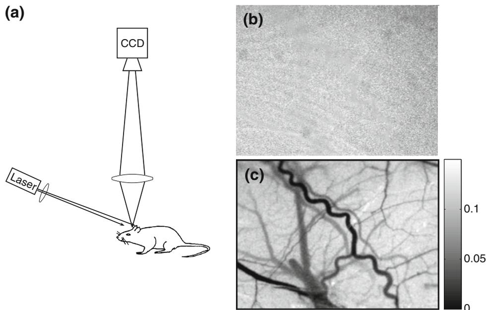
**FIGURE 1.** (a) Basic LSCI setup consisting of a laser diode and camera. A raw speckle image of the rat cortex, taken through a thinned skull, contains seemingly little information (b). However, when the speckle contrast is calculated using a sliding window (c), a tremendous amount of information is revealed about the motion of the scattering particles in the sample.
