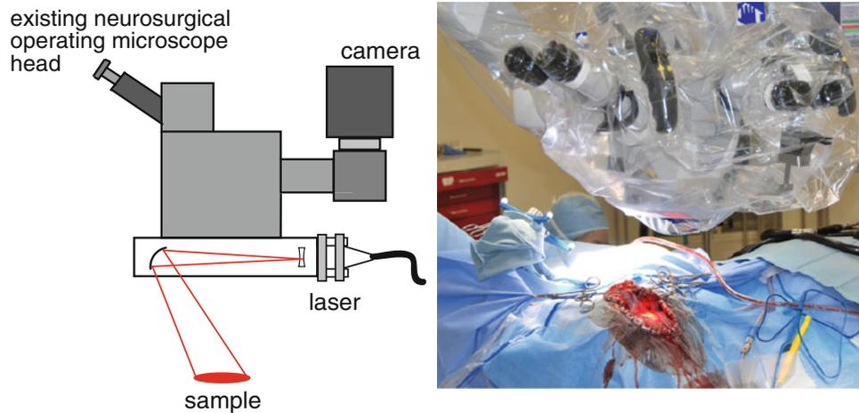
**FIGURE 4.** Schematic and photograph of neurosurgical operating microscope adapted for real-time speckle imaging of blood flow during neurosurgery. A commercially available laser illuminator was fitted with a laser diode (660 nm) and a camera was attached to an existing camera port on the microscope, which enabled all of the instrumentation to be contained within the surgical drape.
