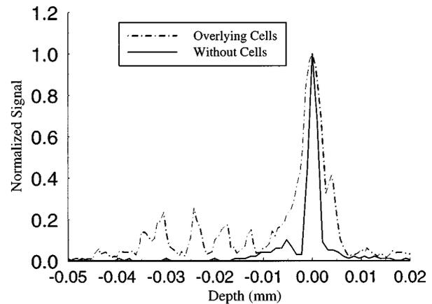
**Fig. 7** Axial scan through a 1.33/1.51 index mismatch with and without overlying cells. The data have been normalized to the peak signal value.
