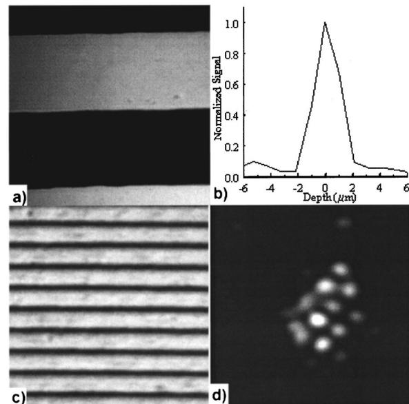
**Fig. 2** (a) Confocal image of the 500 lines/in. grating in which each line is  $25\ \mu\text{m}$  wide. (b) Plot of intensity versus depth relative to the focal plane for a mirror translated through the focal plane. (c) Confocal image of a 300 lines/mm grating where each line is separated by  $3.3\ \mu\text{m}$  and (d) a cluster of  $1\ \mu\text{m}$  diameter polystyrene microspheres.
