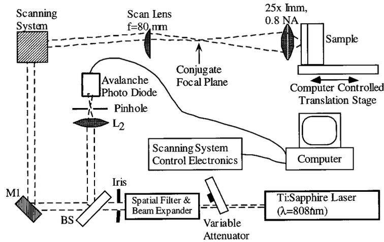
**Fig. 1** Schematic of the confocal microscope built to acquire cellular images from reflected light.
