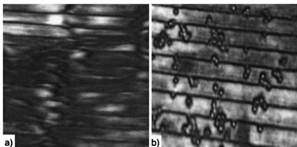
**Fig. 6** 300 lines/mm grating under (a) multiple layers of cells and (b) two optical depths of scattering from 1  $\mu\text{m}$  polystyrene spheres.
